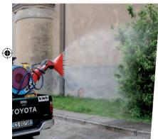
The perfect and uniform micronization produced using a unique type of pneumatic nozzle, with a large diameter (4 mm), and fade-free functionality, no wear, no clogging, no maintenance.
